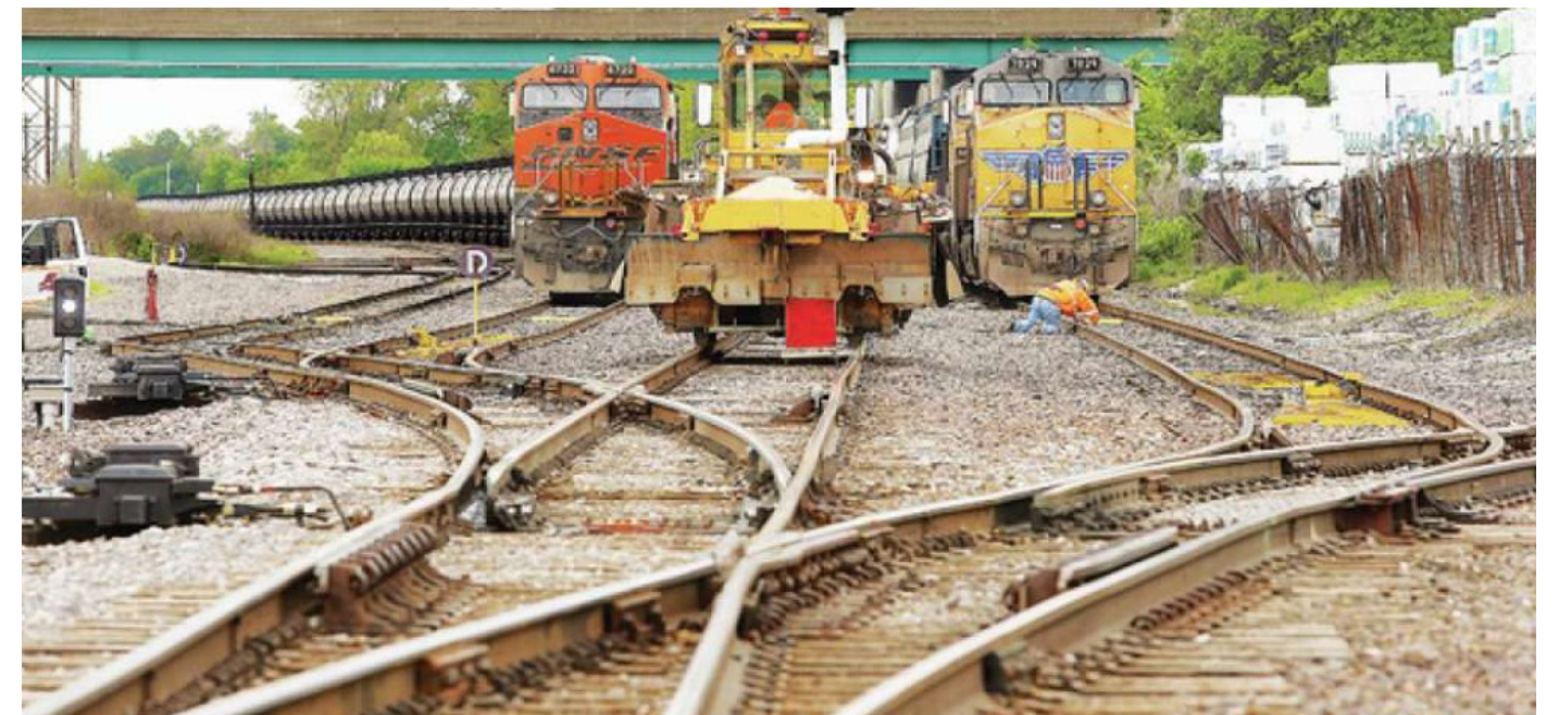
An average of 66 trains pass through the Lenox Tower interlock, which is located at the intersection of four railroads: Union Pacific, Canadian Pacific Kansas City, Norfolk Southern, and Alton & Southern. Movements were restricted by diverging turnouts and a specialty track switch known as a single slip switch.
