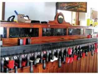
Right (Top): The Lenox Tower's interior housed the operator's office and the interlocking equipment, which consisted of the interlocking machine and track model board. The Lenox Tower was one of the last three manually operated interlocking plants in the St. Louis area in Illinois.
