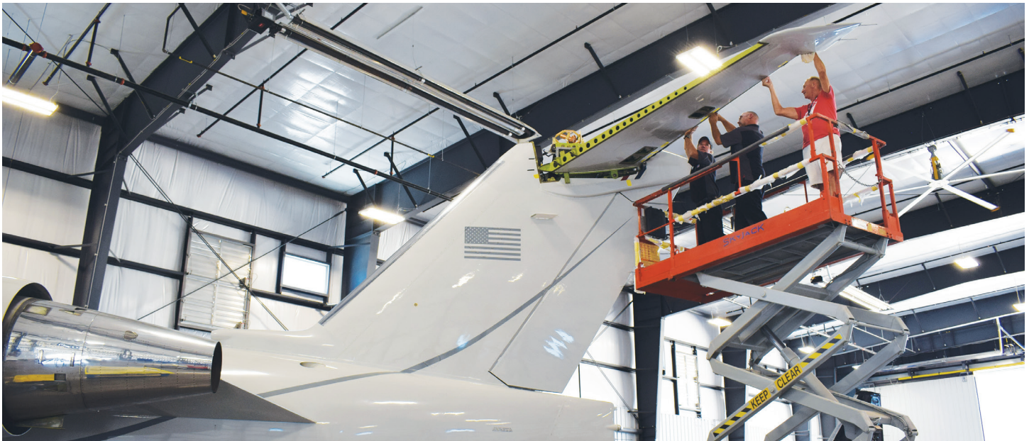
Team work: assembling horizontal stabilizer and elevator tab on t-tail
